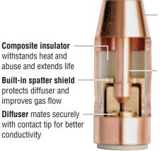
Threaded nozzles keep contact tips centered and fixed at desired position for better weld placement and less spatter
